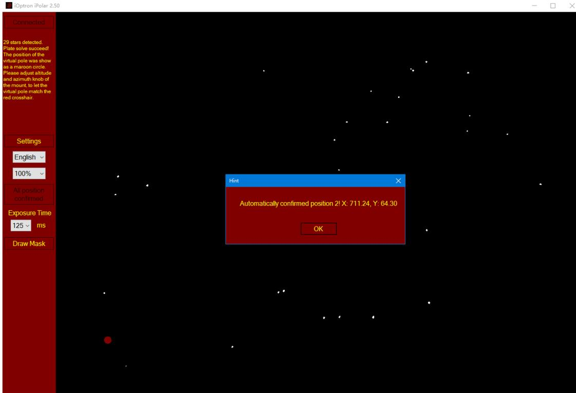
The software will display the virtual pole with a maroon circle and camera center a red cross.
