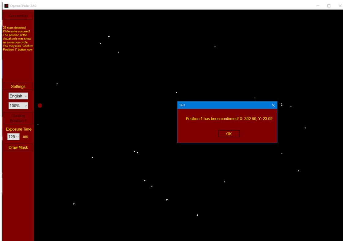
If you are lucky enough that the RA axis is aligned to the Pole, you'll see both the cross (camera center) and the circle (virtual pole)! Otherwise, follow the on-screen instruction to use hand controller or iOptron Commander to rotate the mount in RA. The software will confirm the **Position 2** automatically during rotation. The closer the RA axle is to the pole, the smaller the rotation angle is needed. Click **OK** to close the position 2 confirmation window.
