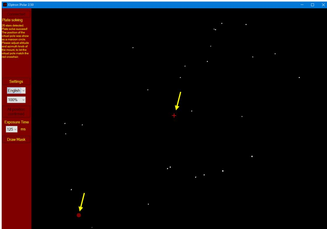
If the virtual pole is far away from the RA axis and can not be displayed inside the screen, an arrow will show where it is located.
