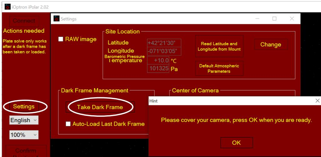
You may skip Take Dark Frame by click on Load Last Dark Frame if the camera was disconnected short while ago. We recommend to take the dark frame when performing polar align. If the software does not plate solve, please retake the Dark Frame.
